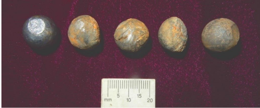
Figure 17. Unfired 0.626-inch ball, fired balls l to r fired at 905 f/s, 960 f/s, 960 f/s, and 1090 f/s. All balls recovered at 100 yards in sand and soil backstop. Note third ball from the left passed through a pine 4x4 target frame upright and the fourth ball from left also struck the edge of the pine target frame before embedding in the backstop.
