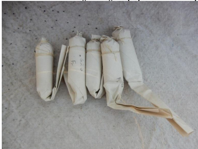
Figure 6. Completed cartridges with notes on the laid paper body denoting ball size and intended firearm.
