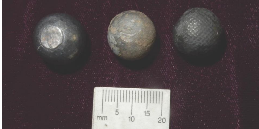
Figure 15. Unfired 0.626- inch ball, 0.626 ball fired at 775 f/s recovered from a soil and sand backstop at 100 yards and a 0.626 ball fired at 785 f/s and captured in ballistic gel at 25 yards after passing through 30 inches of gel. Note ramrod mark on second ball and fabric impressions on third ball.
