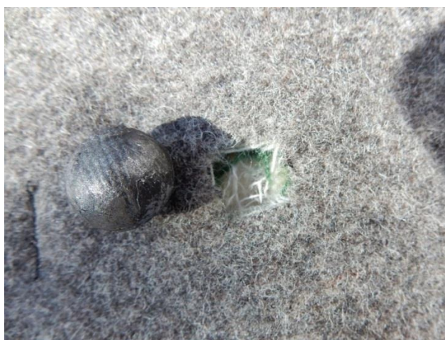
Figure 8. A fabric impressed .69 diameter ball fired from the British 1756 Long Land Pattern musket with 75 grains of powder at 25 yards. The fabric impressions resulted from passing through the simulated uniform clothing.
