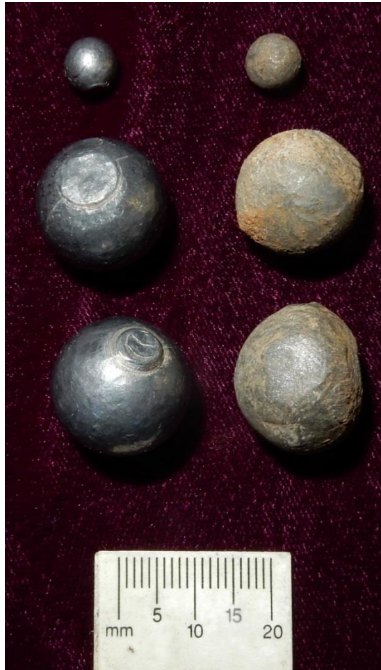
Figure 16. Top row: Unfired 0.282-inch buckshot and fired 0.282-inch buckshot at 865 f/s. Second row: Unfired 0.626-inch ball and fired 0.626-inch ball at 865 f/s. Third row: Unfired 0.69-inch ball and fired 0.69-inch ball at 870 f/s. Note each recovered in the sand and soil backstop at 100 yards.
