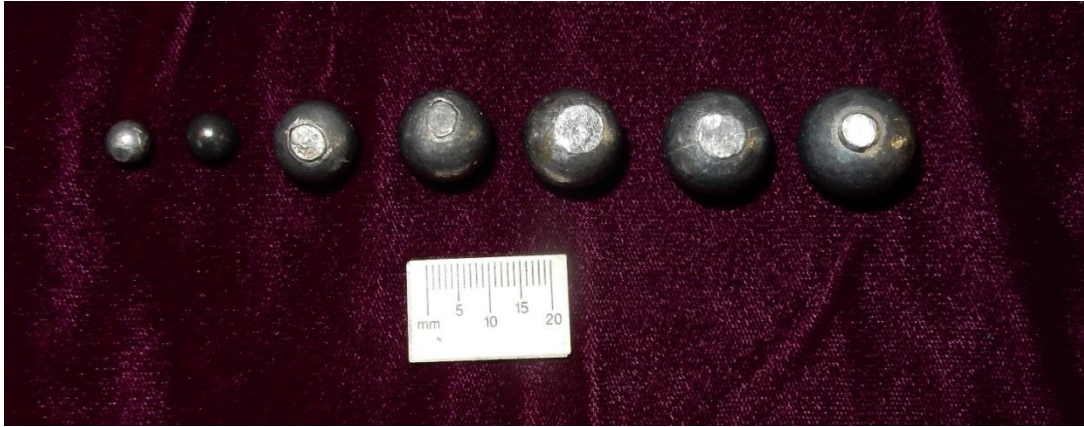
Figure 3. Unfired cast lead balls used in the experimental firing. L to R, .315 buckshot, .282 buckshot, .520 ball, .580 ball, .626 ball, .663 ball, and .69 ball.
