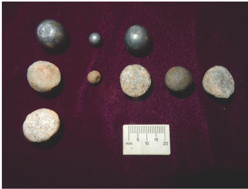
Figure 18. Left column, unfired 0.626-inch ball, fired 0.626 balls at 1110 f/s and 1175 f/s, both found in sand and soil backstop. Second column, unfired 0.282 buckshot and fired 0.282 buckshot at 1110 f/s found in sand and soil backstop. Third column, unfired .580-inch ball and fired 0.580 ball at 1135 f/s found in sand and soil backstop. Fourth column, 0.580 ball fired at 1155 f/s, and Fifth column, 0.580 ball fired at 1170 f/s and found in soil and sand backstop. All balls recovered at 100 yards.
