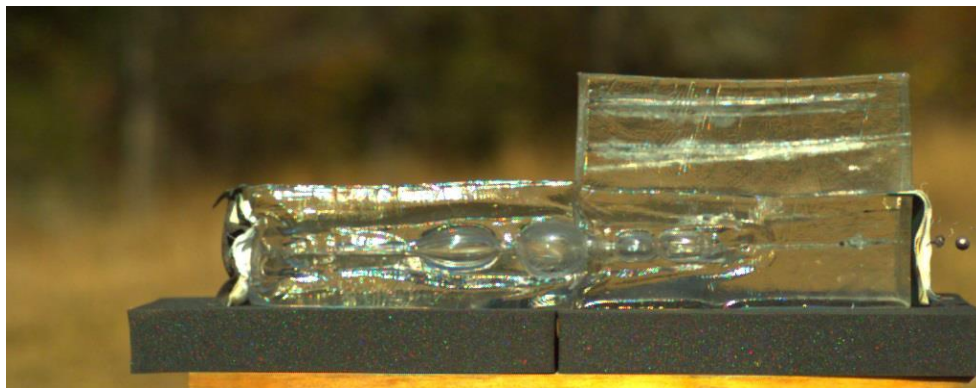
Figure 7. A .69 diameter ball fired from a British 1756 Long Land Pattern musket exiting 32 inches of gelatin. Note the initial wound cavity, bits of cloth in the wound cavity on the right and a larger piece of cloth exiting the block behind the ball.
