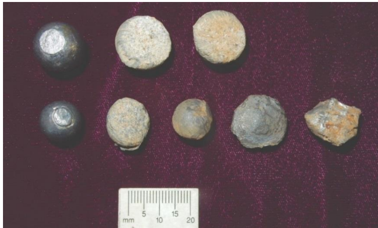
Figure 19. Top row, Unfired 0.626-inch ball, fired 0.626 ball at 1205 f/s and found in sand and soil backstop, fired 0.626 ball at 1215 f/s which nicked the target frame post and was found in the sand and soil backstop. Bottom row, Unfired 0.520-inch ball, fired 0.520 ball at 1215 f/s that hit oak palisade paling and ricocheted back into sand and soil backstop, fired 0.520 ball at 1250 f/s which hit a pine palisade paling and ricocheted back into sand and soil backstop, 0.520 ball at 1240 f/s that struck an oak palisade paling and fell to the ground below the fence, and 0.520 ball fired at 1285 f/s that went through a 4x4 pine target frame upright and was recovered in the sand and soil backstop. All balls found at 100 yards.
