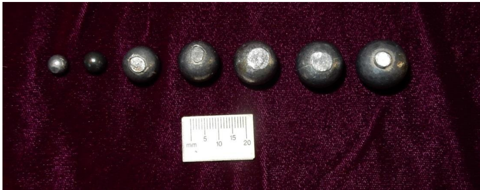
Figure 13. Unfired buckshot and bullet examples as used in the live fire experiments. l to r – 0.28-inch buckshot, 0.31-inch buckshot, 0.520-inch ball, 0.580-inch ball, 0.626-inch ball, 0.662-inch ball, and 0.69-inch ball.
