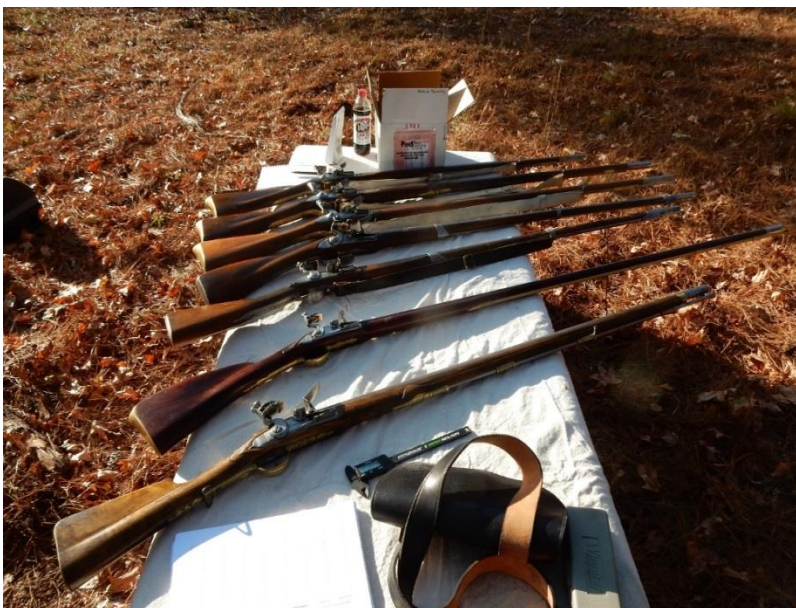
Figure 1. The firearms used in the live fire experiment. Top to bottom, British Artillery Carbine, British 1742 Long Land Pattern musket, British 1756 Long Land Pattern musket, French 1728/41 musket, French 1763/66 musket, Thomas Earle fowler, and a Potsdam 1740 musket.
