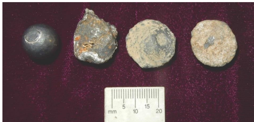
Figure 21. Unfired 0.580-inch ball and fired balls, second – fired at 1415 f/s and struck oak palisade paling and found in sand and soil backstop below fence, third – fired at 1435 f/s and found in sand and soil backstop, fourth – fired at 1480 f/s and found in sand and soil backstop. All balls recovered at 100 yards.
